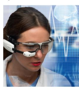
With integrated GPS, gyroscope and compass systems, apps can sense your location and even the direction and angle of your current view for highly accurate environmental awareness. Voice, button press, and gesture controls give the user a variety of ways to navigate the M100 in almost any working environment.
